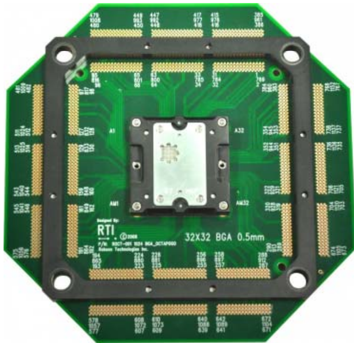
Handler Interface Board(HIB)
